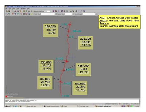
Figure 3. PARAMICS I-710 network and truck counts based on 2005 data.
