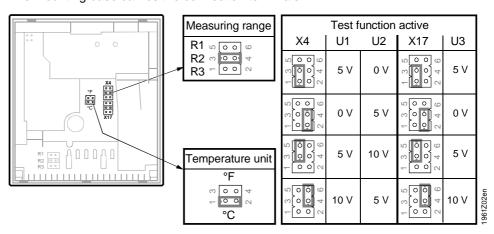
The setting elements can be accessed after removing the mounting base.
