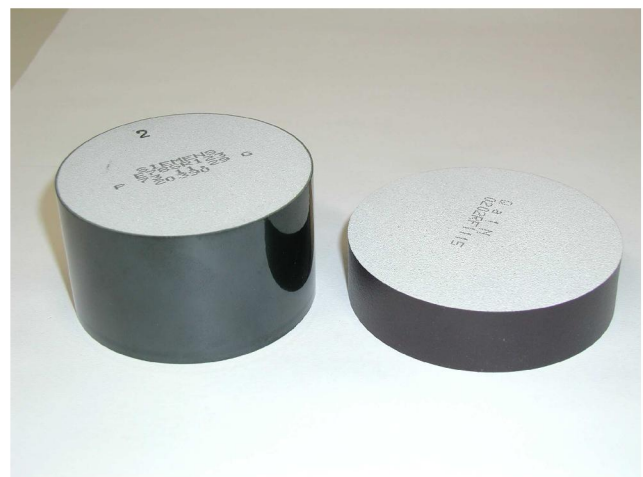
Fig. 3. Comparison of conventional and High Voltage Gradient metal oxide resistors (same rated voltage)
