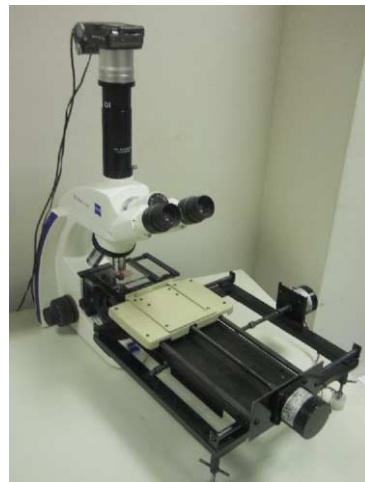
Figure 1– Camera coupled to microscope, focusing a bone tissue sample disposed on the XY-table.
