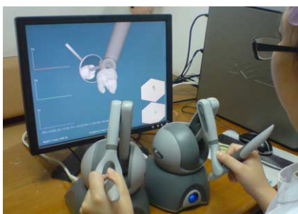
Figure 1 - A dentist performed access opening to the root canals with a haptic virtual reality simulator
