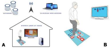
Figure 1. Schematic of main components of the telehealth step training system including sensor mat paired with low-cost PC connected to TV (A). Representation of the modified step training game (B).
