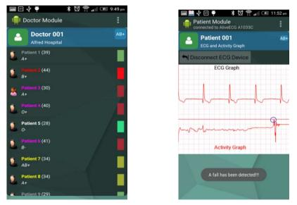
Figure 2. (a) Doctor's portal showing a list of patients; and (b) Patient's portal showing the ECG graph and the magnitude of three-dimensional acceleration. It follows from the graph that the magnitude of acceleration crosses the threshold  $\tau$  during the fall.
