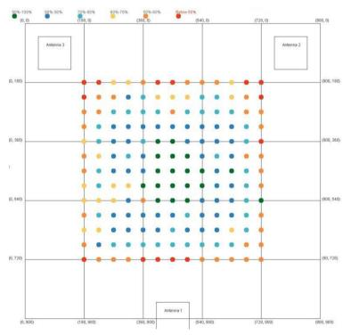
Figure 3. Accuracy distribution of tracking a passive RFID tag over various locations in the localisation area.
