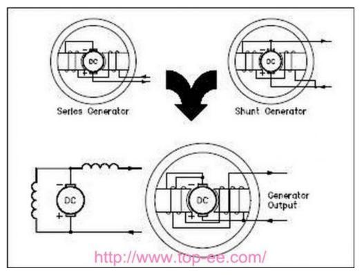
Among various types of DC generators, the compound wound DC generators are most widely used because of its compensating property. Depending upon number of series field turns, the cumulatively compounded generators may be over compounded, flat compounded and under compounded. We can get desired terminal voltage by compensating the drop due to armature reaction and ohmic drop in the in the line. Such generators have various applications.
