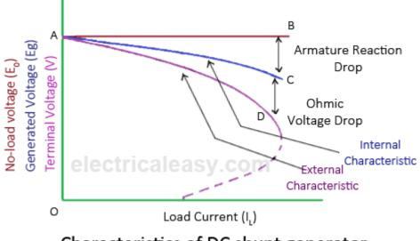
Characteristics of DC shunt generator
