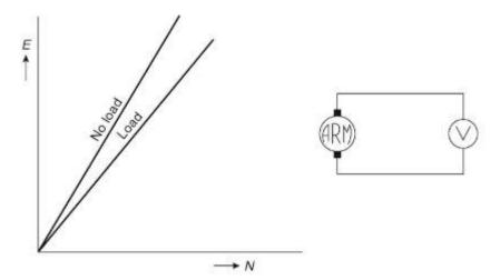
If a sensitive voltmeter is used, i.e. one requiring negligible current, generator output will be so small that the armature drop ( $I_aR_a$ ) will be negligible. The load terminal voltage is nearly equal to the generated e.m.f  $E_g$ .
