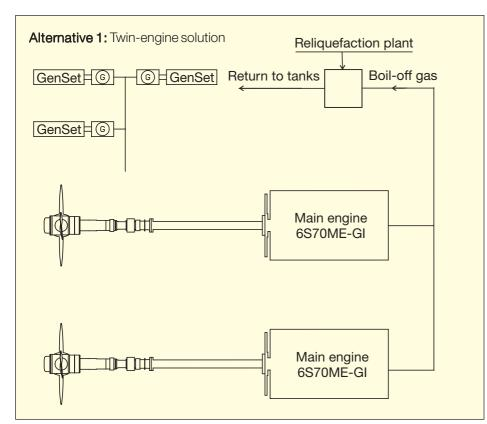
Fig. 13: LNG carrier propulsion systems
