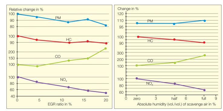
Fig. 20: Emission parameters at 75% load at various EGR ratios
