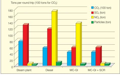
Fig. 12: Round trip emissions, 135,000 m<sup>3</sup> LNG carrirer
