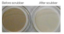
Fig. 21: PM on filters before and after scrubber
