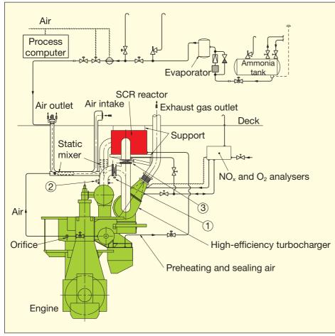
Fig. 24: SCR system layout
