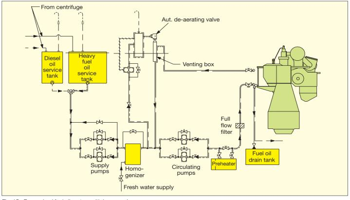
Fig. 15: Pressurised fuel oil system with homogeniser
