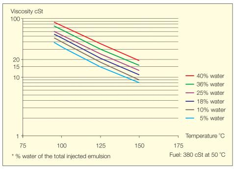
Fig. 16: Viscosity versus water percentage
