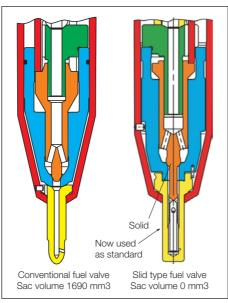
Fig. 6: Fuel valves for K98MC
