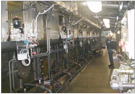
Fig. 9: 12K98MC-C with Alpha Lubricator System
