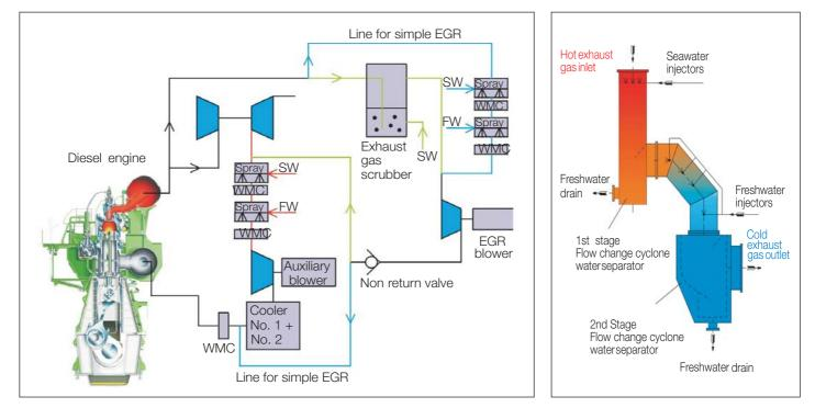
Fig. 17: Schematic design of EGR and HAM systems application on the 4T50ME-X engine
