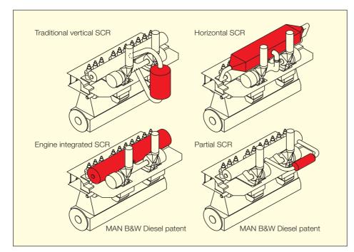
Fig. 26: Alternative SCR configurations
