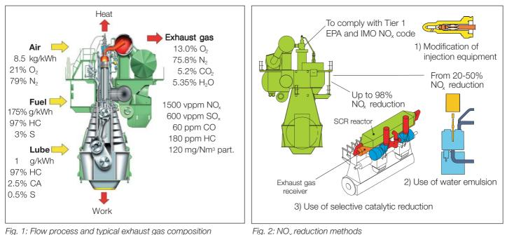
Fig. 1: Flow process and typical exhaust gas composition
