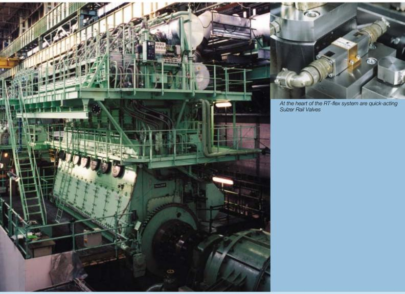
Sulzer 7RT-flex60C engine during shop test
