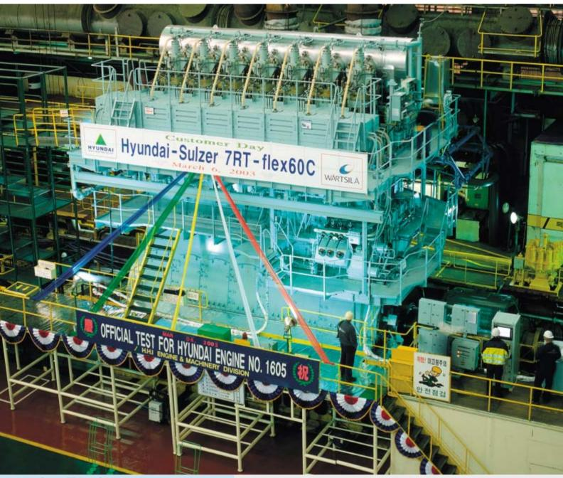
Sulzer 7RT-flex60C engine during shop test
