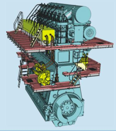
The main elements of the RT-flex system can be seen in yellow: the supply unit with fuel and servo oil pumps, the rail unit alongside the cylinders, and the servo oil filter on the other side.
