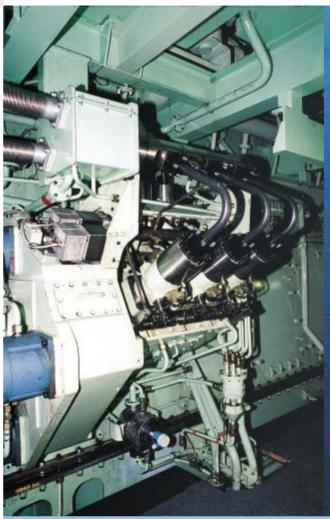
Supply unit of the 7RT-flex60C with fuel pumps on the right and the servo oil pumps on the left
