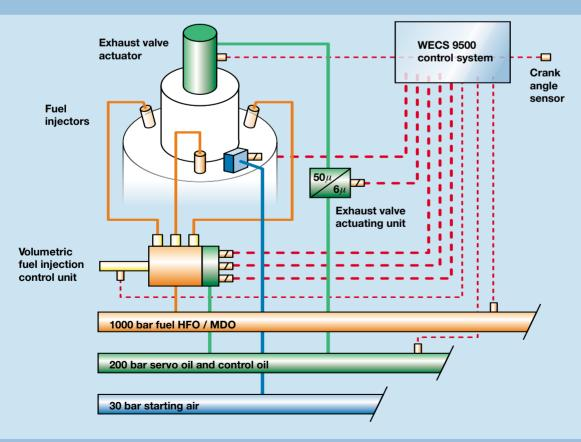
Sulzer RT-flex engines have electronically-controlled common-rail systems for fuel injection and exhaust valve actuation
