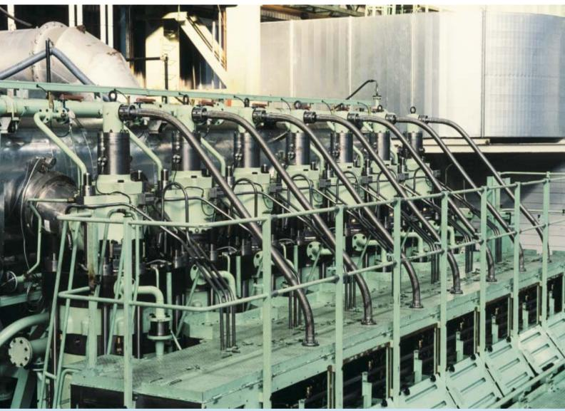
Cylinder tops of the 7RT-flex60C with rail unit open at the side for access
