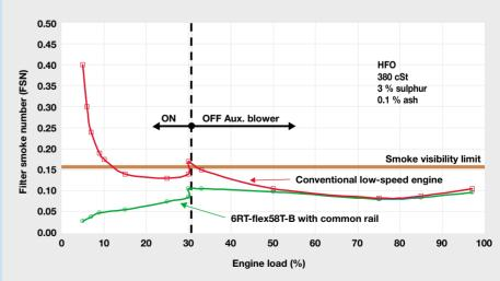
Smoke measurements from the sea trials of the first Sulzer RT-flex engine demonstrate the smokeless operation of RT-flex engines compared with conventional low-speed engines
