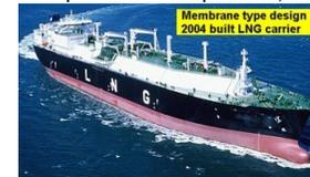
The shape of the LNG Carrier is quite unmistakable, with the shape of the Moss tanks (which are like enormous spherical thermos flasks !) visible along the deck, which has led to the nickname of "Dinosaur Eggs Carriers". An alternative design is known as the "membrane" type, which allows for a more standard shape of vessel without the "eggs".
