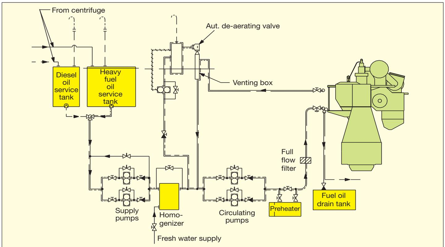
Fig. 15: Pressurised fuel oil system with homogeniser
