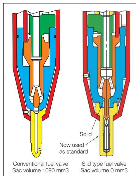
Fig. 6: Fuel valves for K98MC
