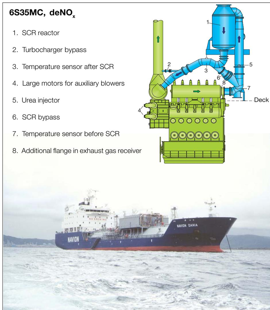
Fig. 29: *M/V Navion Dania* with SCR catalytic reactor installed
