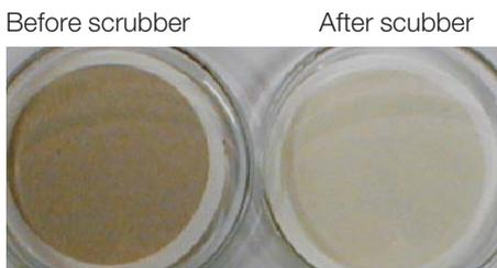
Fig. 21: PM on filters before and after scrubber
