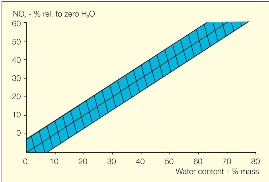
Fig. 14: Typical measured NO<sub>x</sub> reductions when using emulsified fuels
