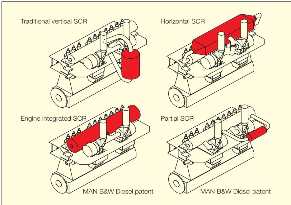
Fig. 26: Alternative SCR configurations
