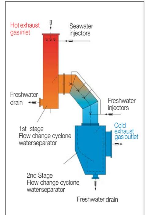
Fig. 18: Design principle of the simple EGR unit
