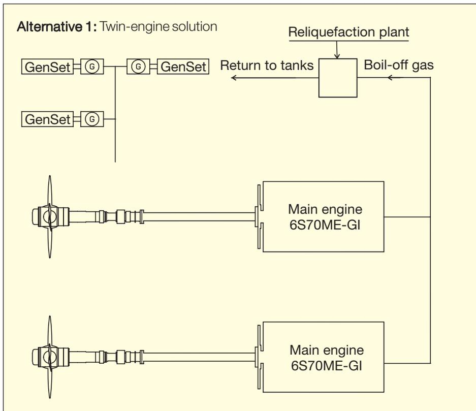
Fig. 13: LNG carrier propulsion systems
