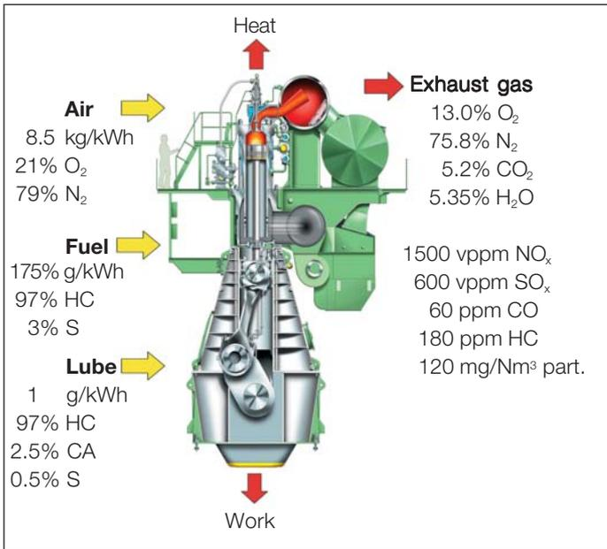
Fig. 1: Flow process and typical exhaust gas composition
