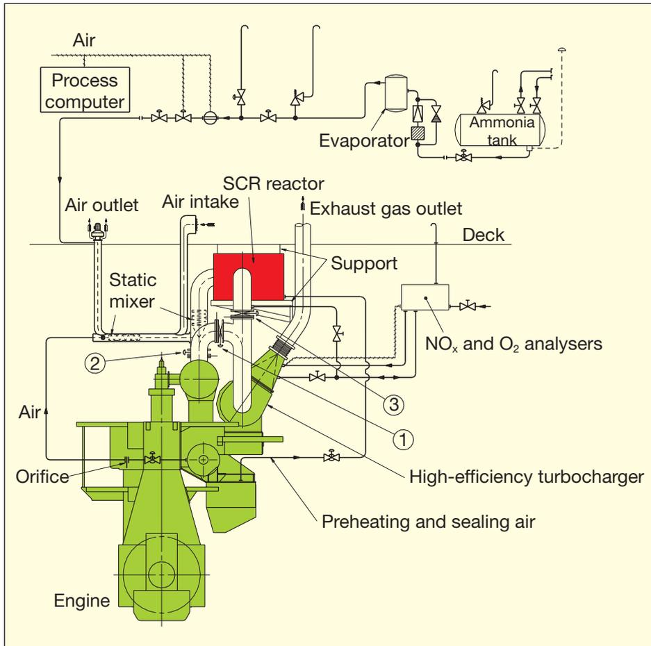
Fig. 24: SCR system layout
