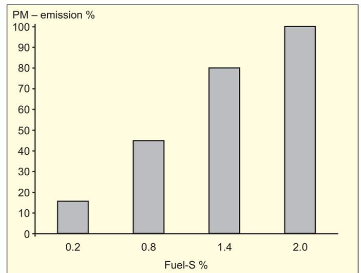
Fig. 8: Emission of particulates as a function of fuel sulphur content
