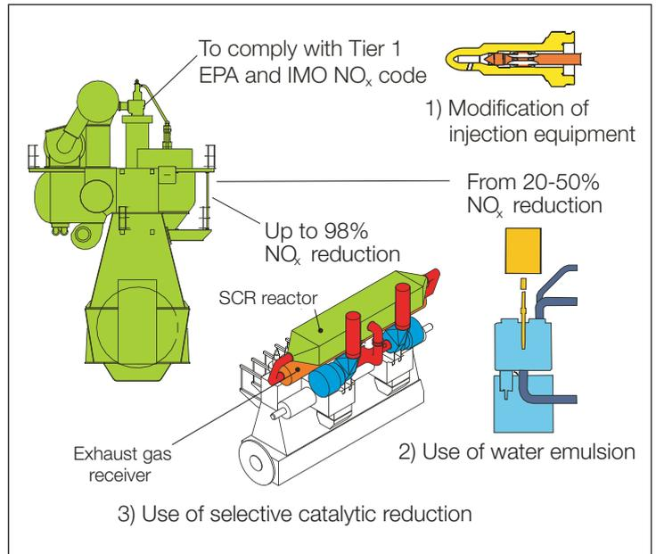
Fig. 2: NO<sub>x</sub> reduction methods
