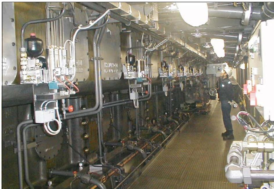
Fig. 9: 12K98MC-C with Alpha Lubricator System
