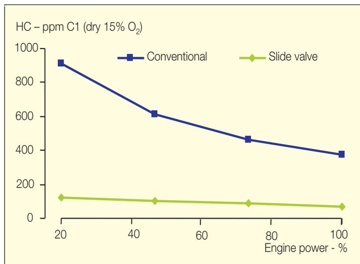
Fig. 7: Hydrocarbon emission, fuel valve comparison – 7S50MC-C
