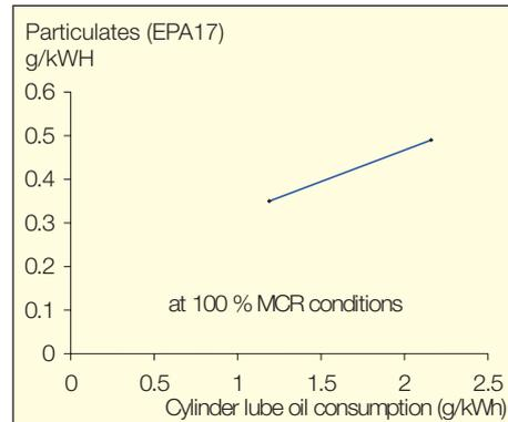
Fig. 10: Particulate emission as a function of cyl. lube oil consumption
