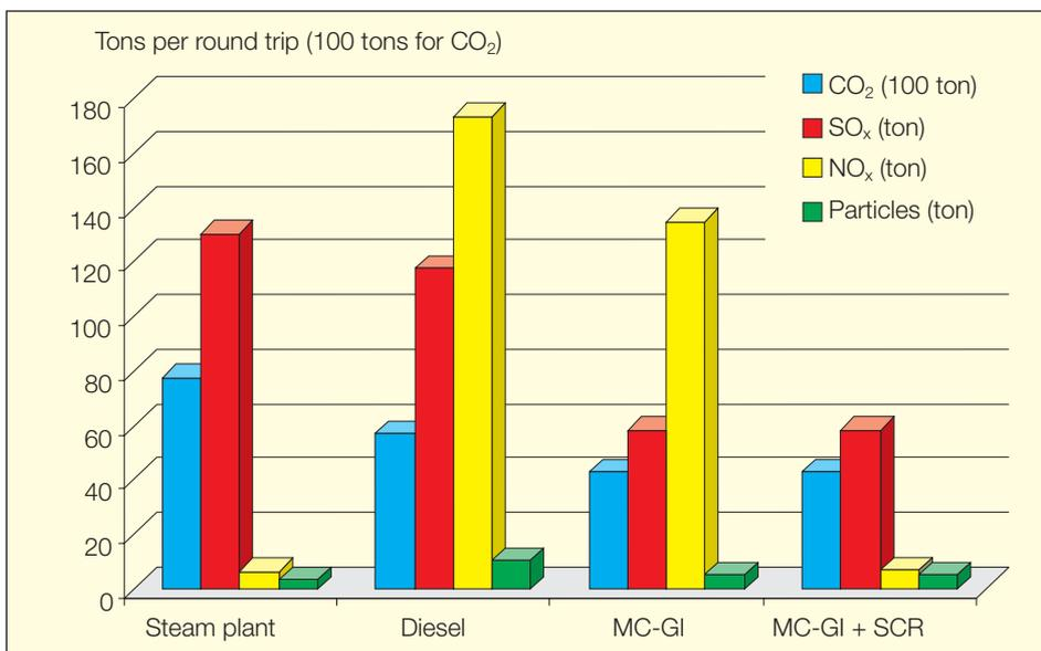
Fig. 12: Round trip emissions, 135,000 m<sup>3</sup> LNG carrier
