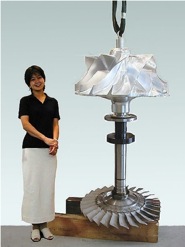
Fig. 4 Rotor from an ABB TPL91-B turbocharger
