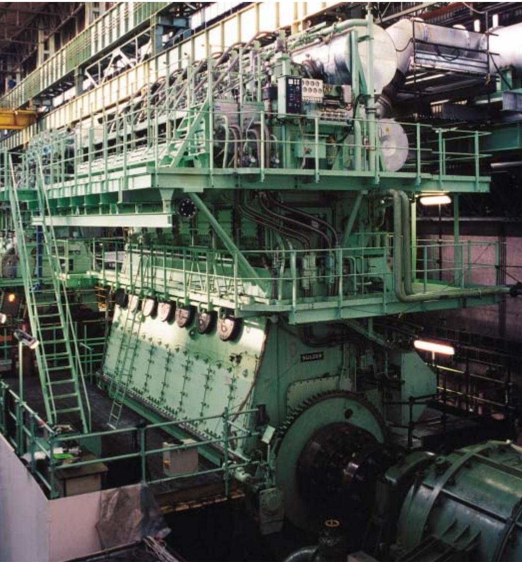
*Sulzer 7RT-flex60C engine during shop test*
