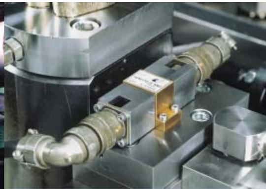
*At the heart of the RT-flex system are quick-acting Sulzer Rail Valves*
