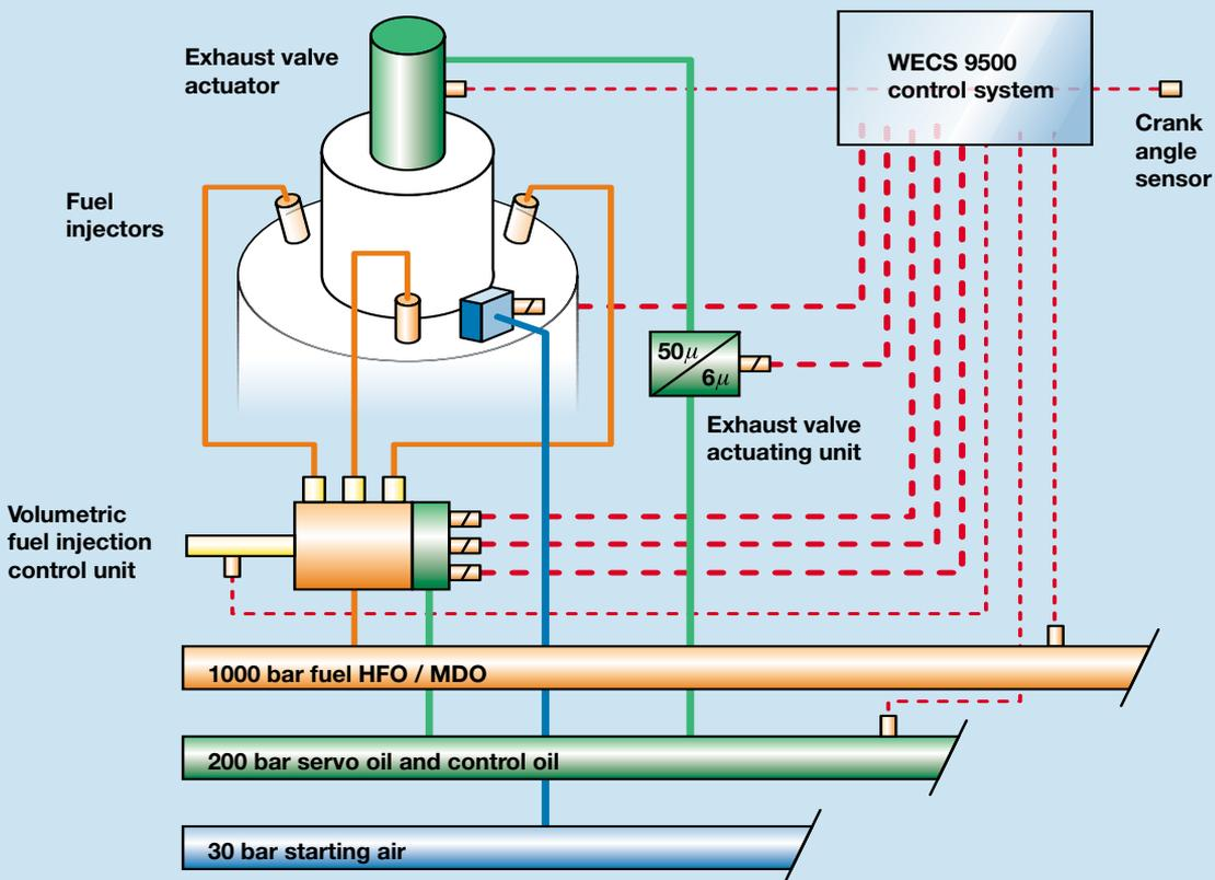
Sulzer RT-flex engines have electronically-controlled common-rail systems for fuel injection and exhaust valve actuation
