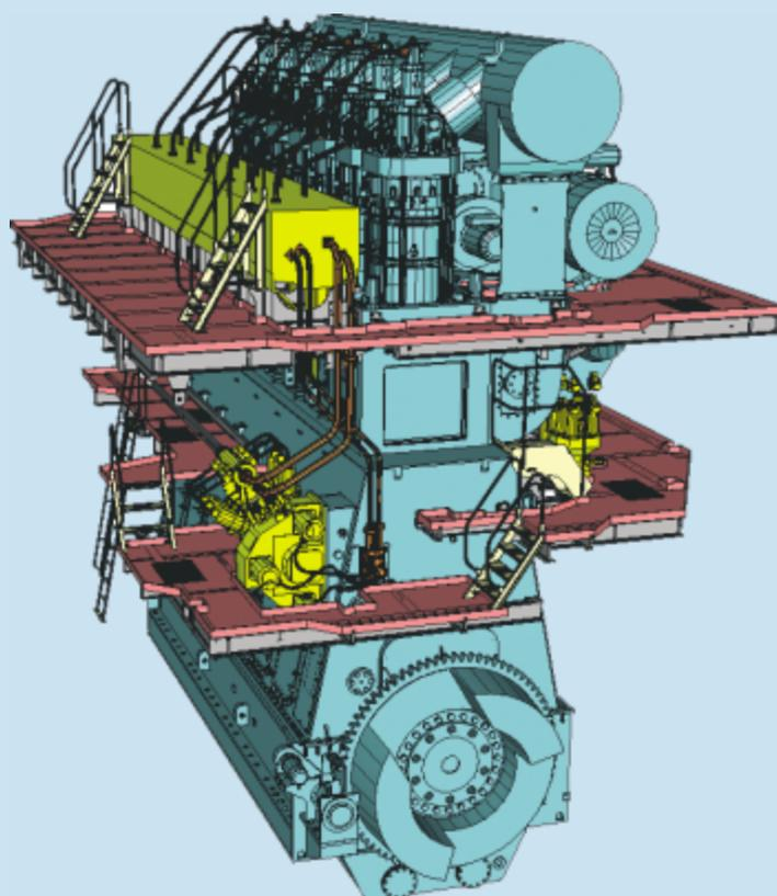
*The main elements of the RT-flex system can be seen in yellow: the supply unit with fuel and servo oil pumps, the rail unit alongside the cylinders, and the servo oil filter on the other side.*
