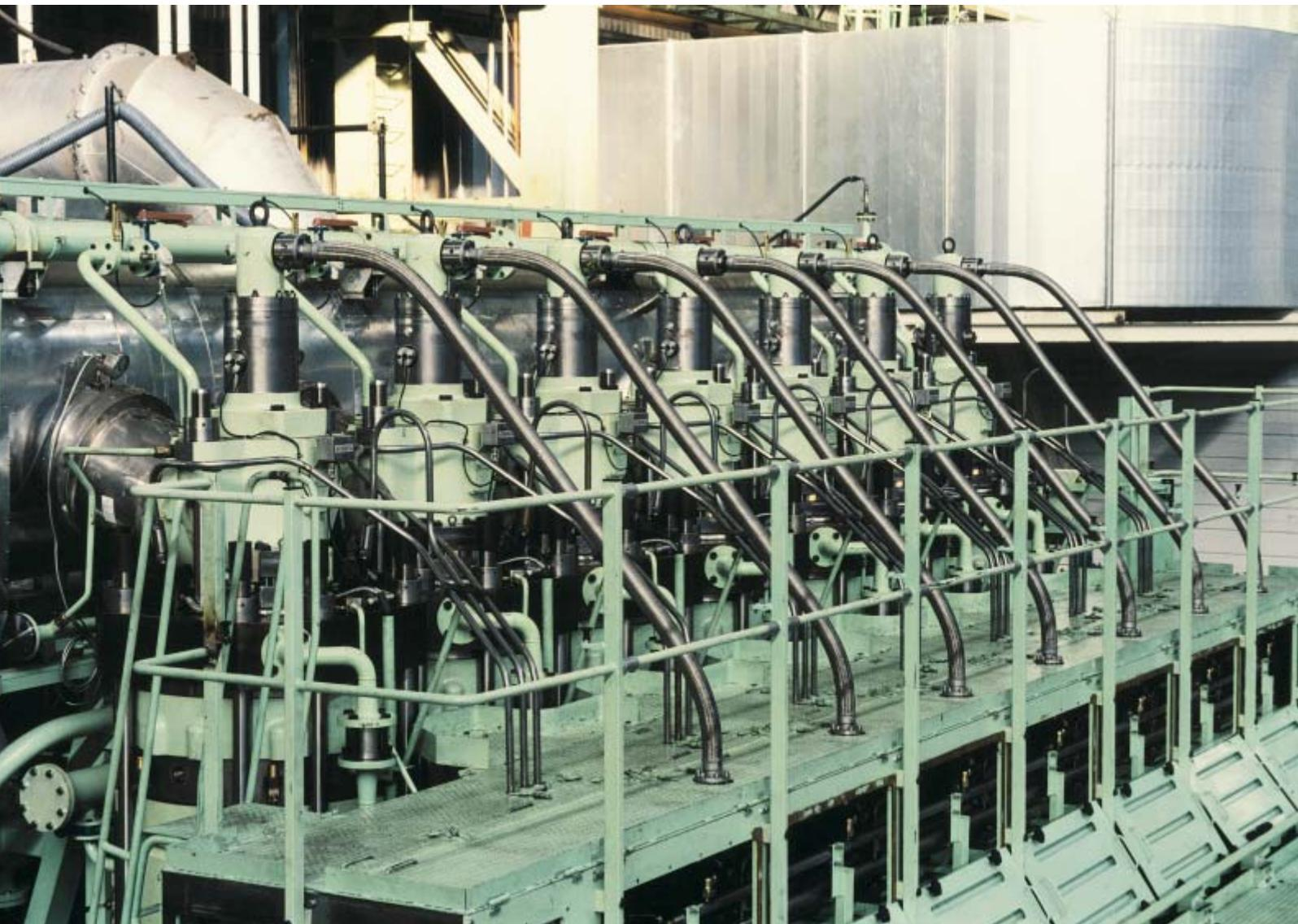
*Cylinder tops of the 7RT-flex60C with rail unit open at the side for access*
