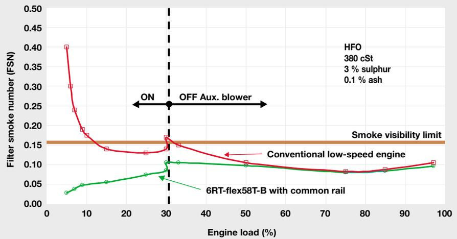
Smoke measurements from the sea trials of the first Sulzer RT-flex engine demonstrate the smokeless operation of RT-flex engines compared with conventional low-speed engines
