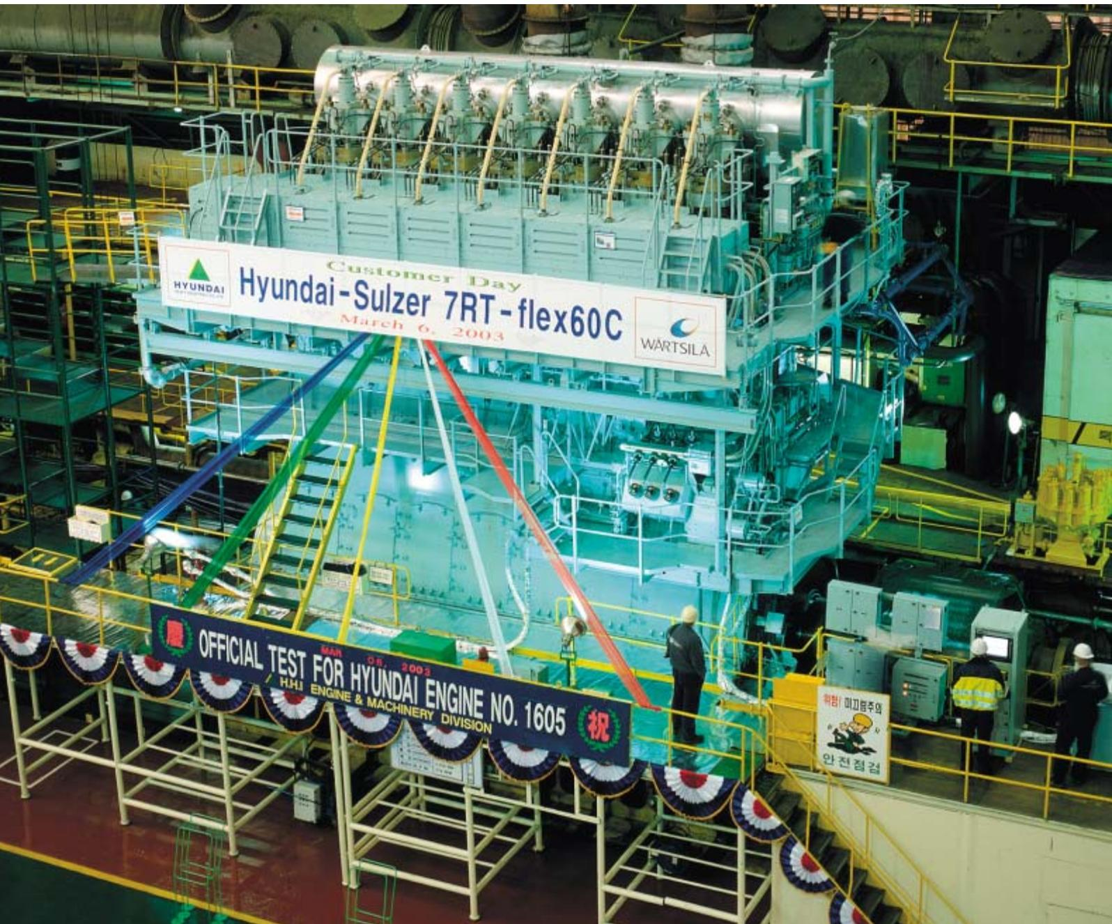
Sulzer 7RT-flex60C engine during shop test
