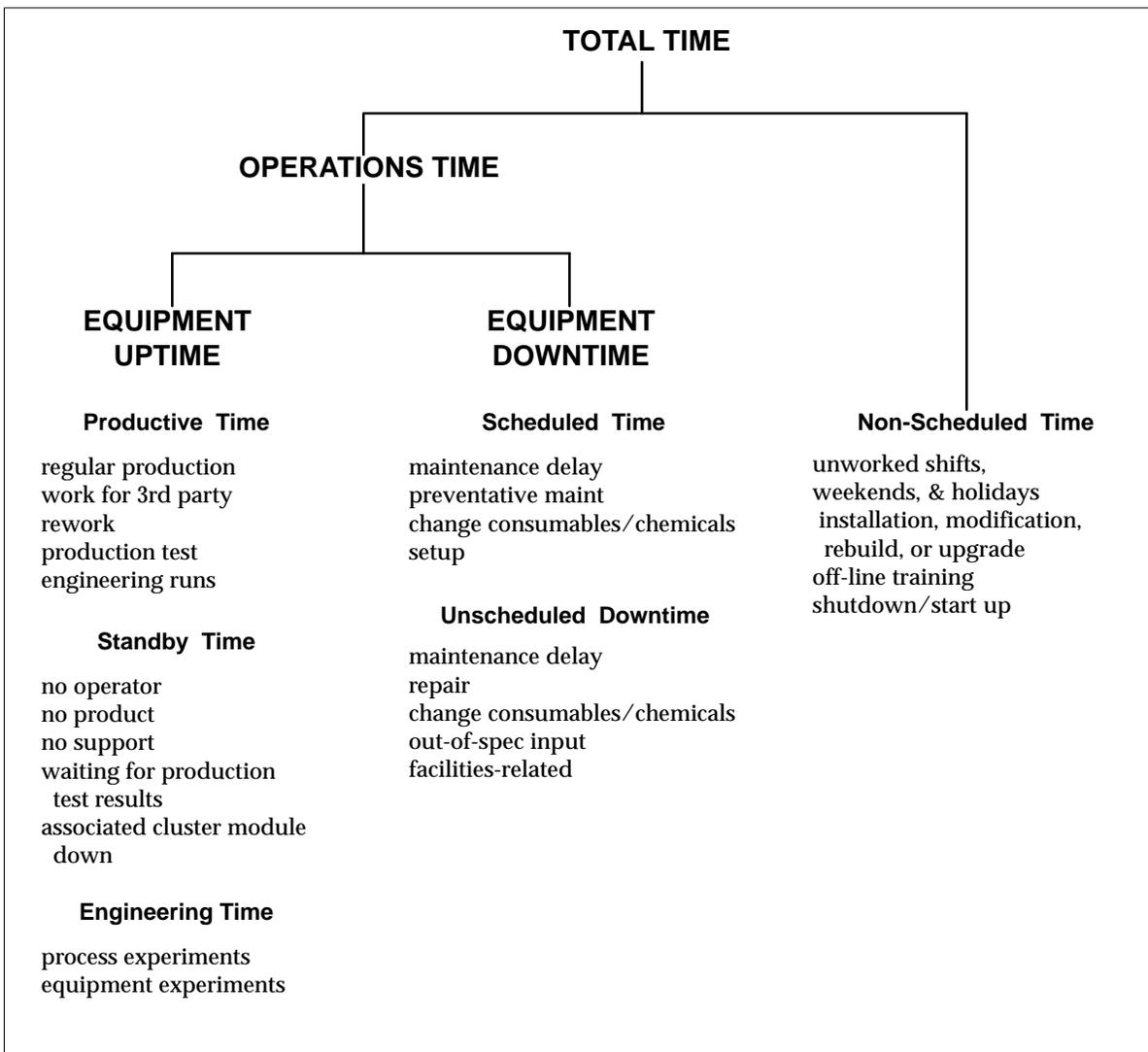
Figure 14. Equipment Allocation of Time (from SEMI E10-92)
