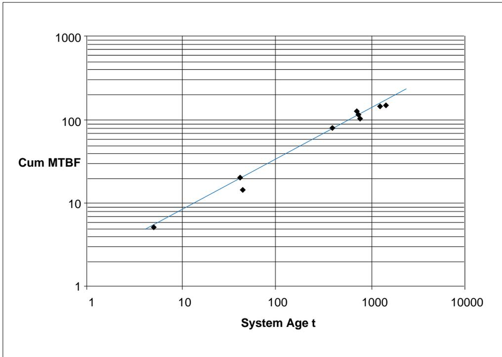
Figure 11. Duane Plot of CUM MTBF vs System Age (time)
