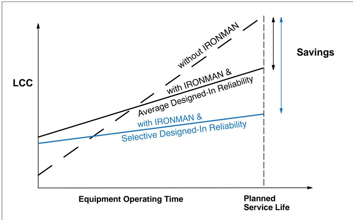
*Figure 5. Impact of IRONMAN Testing and Designed-In Reliability*
