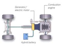
Combustion engine and electric motor are connected in parallel for single or dual usage. Intelligent transmission and clutch systems control the switching between the various operating modes.
