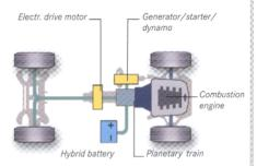
Part of the power from the combustion engine serves to generate power and flows from the generator to two or more electric motors to the drive shafts. The other part is transferred by conventional mechanical means. The planetary train handles the distribution of the electrical and mechanical power.
