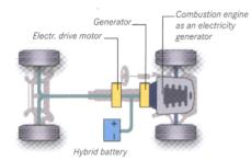
The combustion engine in combination with the generator serves the sole purpose of electricity generation and can run at an emission-optimized speed. The output flows from the generator to two and more electric motors onward to either the drive shafts or directly to the wheel-hub motors.
