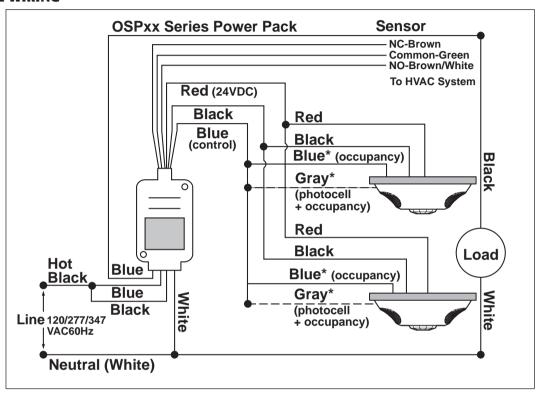
\*When the photocell function is not being used, connect the Blue Occupancy Sensor lead to the Blue Power Pack lead. When using the Photocell function, connect the Gray Occupancy Sensor lead to the Blue Power pack lead—Do not use the Blue Occupancy Sensor lead for the photocell function.
