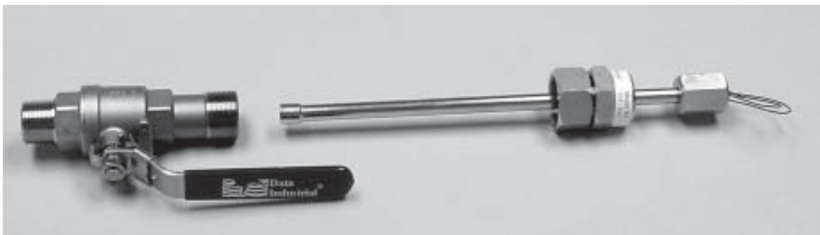
Temperature probe removed from Valve
