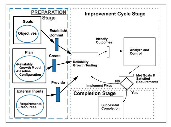
Figure 3. Preparation Stage of IRONMAN
