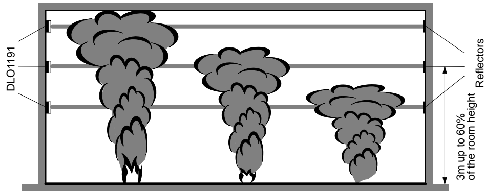
Fig. 17 Detection of smouldering fires in high rooms on different levels
