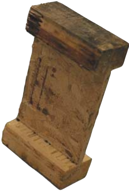
Figure 13-10 To save on materials and cost, the use of composites or engineered wood structural members is becoming popular. Shown here is a typical wood I beam with 2- × 3-in. flanges and a \frac{3}{8} -in. structure board web. In addition to providing a large surface-to-mass ratio, the flanges and web are fastened with glue, which may deteriorate quickly under fire conditions.
