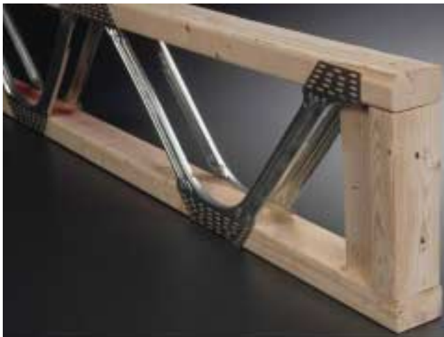
Figure 13-11 A composite truss. Rapid heating will cause the steel to separate from the wood chords.
